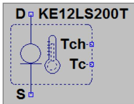
Figure 9. KE12LS200T SiC CLD symbol file: “KE12LS200T.asy”
