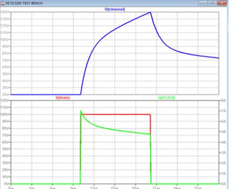
In this example, the CLD is subjected to a 100V square pulse. Self-heating is calculated and the simulated temperature increases up to 139 °C. The dissipated energy value is  $E_{CLD} = 5.3 \text{ mJ}$ .
