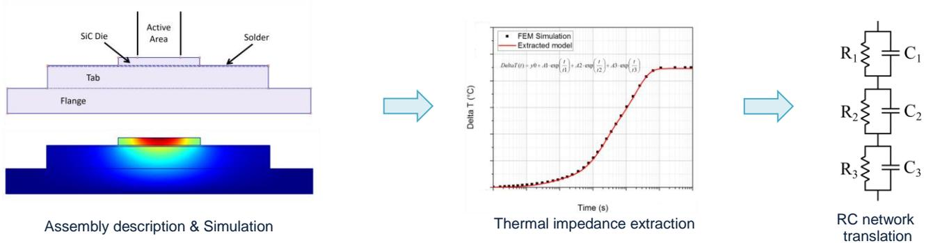
**Figure 4: Thermal impedance extraction**
