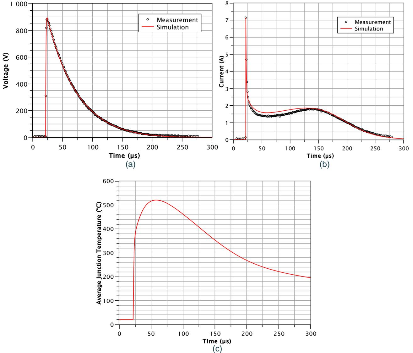
Figure 7: Measured and simulated responses to a 900V 1.2/50µs waveform: (a) Input waveform. (b) Current through CLD. (c) Simulated temperature
