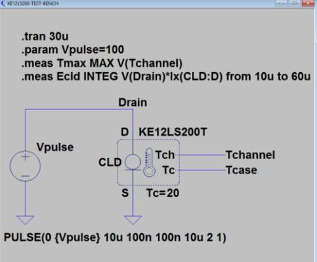
9 Launch the simulation (Simulate -> Run) and add parameters to the plot window
