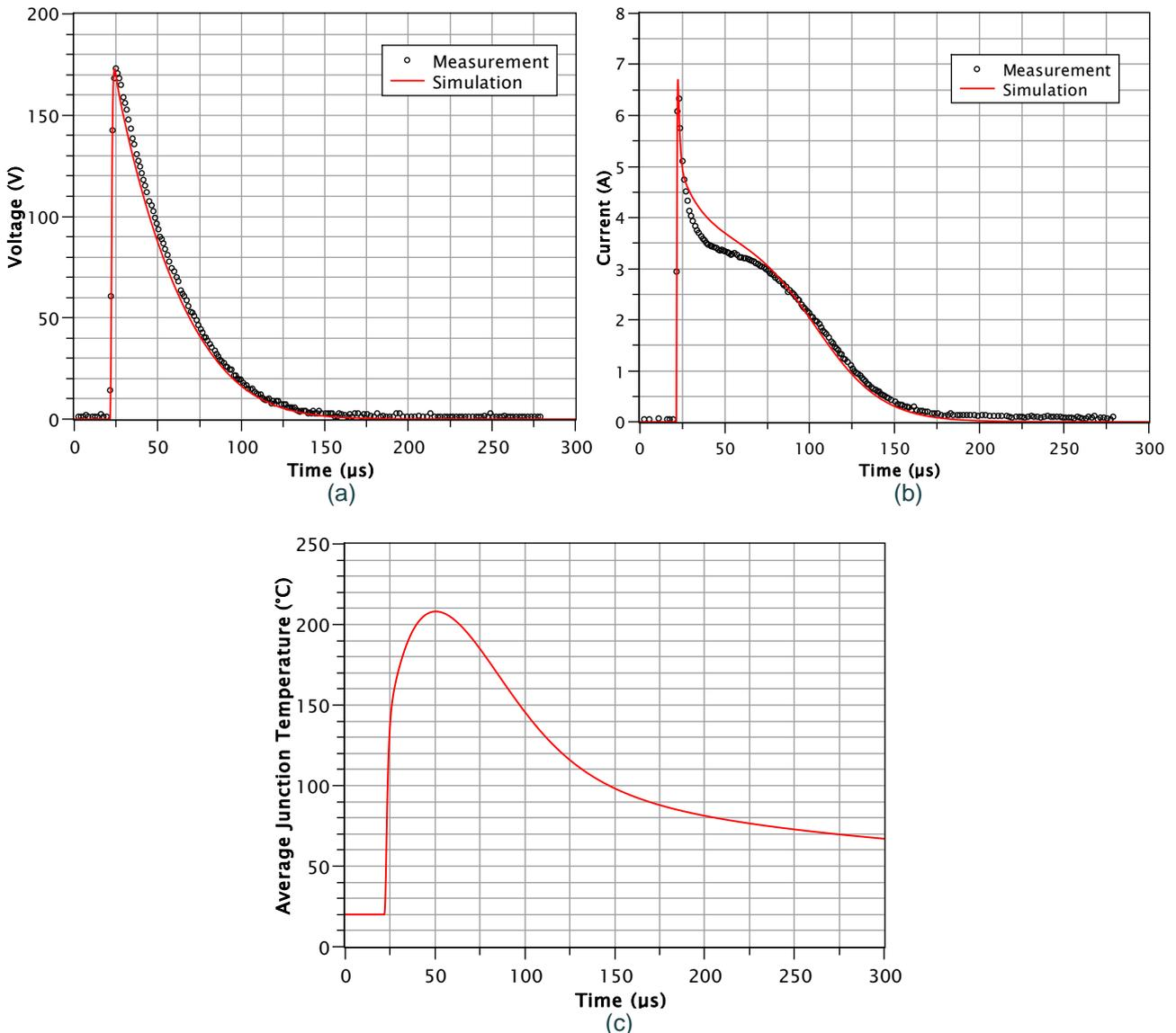
Figure 6: Measured and simulated responses to a 175V 1.2/50 $\mu$ s waveform: (a) Input waveform. (b) Current through CLD. (c) Simulated temperature
