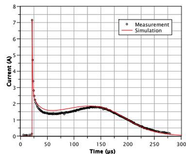
Experimental vs Simulation waveforms
