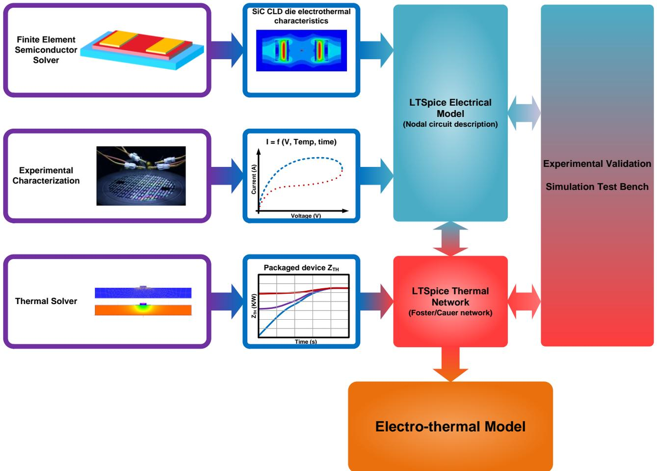
Figure 1. Device modeling procedure.
