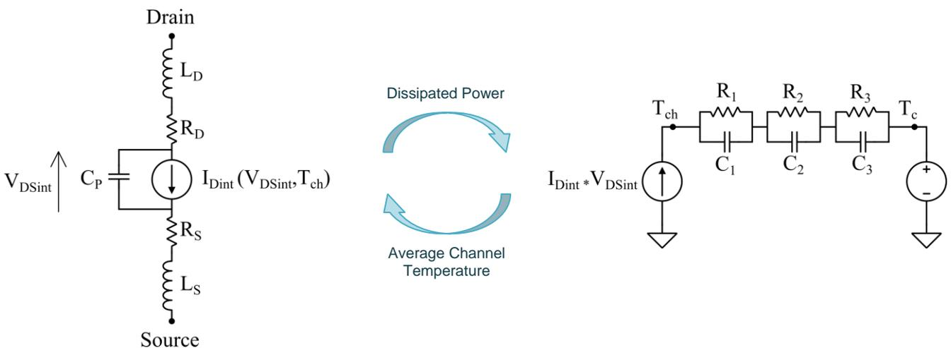
**Figure 2: CLD electro-thermal model circuit diagram**
